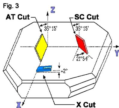
The X Cut tuning fork crystal (Fig. 4) is used in 'Time of Day' timekeeping applications (wrist watches, domestic clocks etc.) because of its natural low frequency of oscillation, very low operating power requirements and low temperature coefficient around 25°C (Fig. 5).
