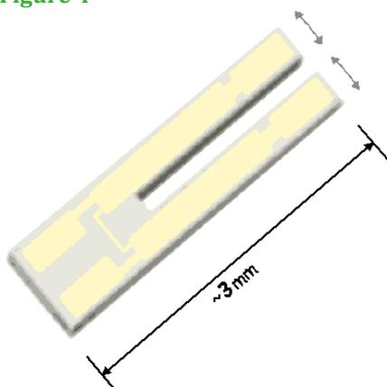
In particular the X Cut tuning fork crystal can be made to oscillate at 32.768kHz which, when digitally divided down by  $2^{15}$ , generates a 1 second square wave, ideal for timekeeping. This same 1 second square wave could
