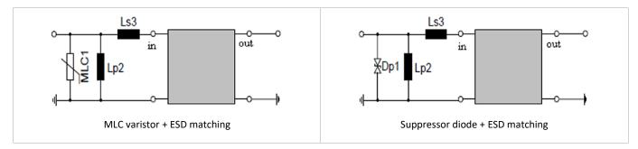
ESD matching" should be added to the filter port, where electrostatic discharge is expected. It predominantly appears at the antenna input of RF receivers. Therefore "ESD matching" should be designed to short circuit or block the ESD pulse.
