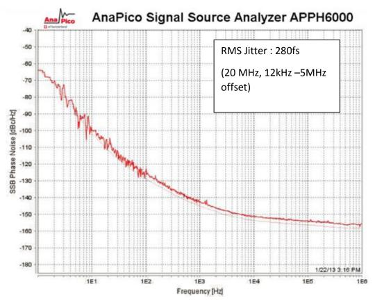
Rakon provides G.8262 compliant TCXOs for synchronous Ethernet applications. Rakon has qualified oscillators for G.8262 which have undergone extensive time domain performance analysis of the clocks at various frequencies. Rakon has worked with numerous timing and synchronisation silicon
